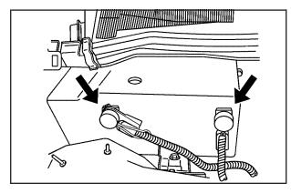
Open the hoods and locate the positive (+) and negative (-) terminal locations of the other vehicle, as well as the positive (+) terminal location on your vehicle's battery. See Engine Compartment Overview on page 356 for more information on the location of the battery.
